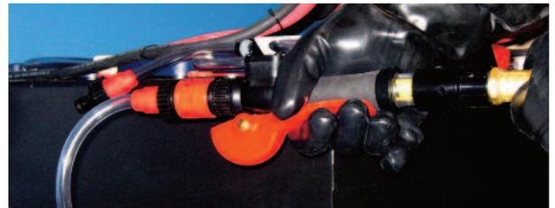
3. Watch the spinner mounted on the Instant Valve Pro. When it stops spinning, the filling is completed (about 15 seconds, usually).
