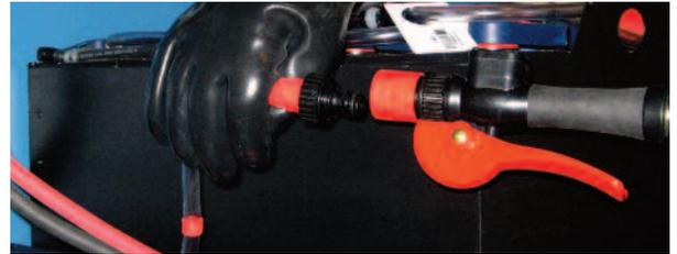
2. Squeeze the lever completely to fill the battery. **Do Not Partially Squeeze the Lever.**
