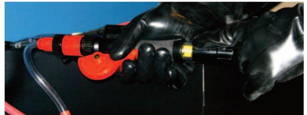
4. Release the lever and then disconnect the Instant Valve Pro from the Water Injector System.
